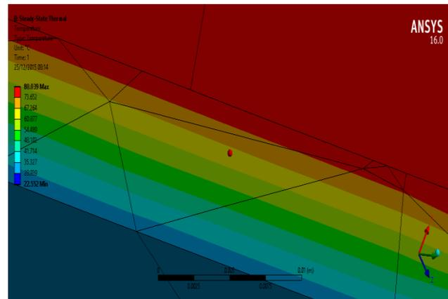
Fig. 5 Cut- section of Temp. Distribution for 5 mm shell wall thickness
