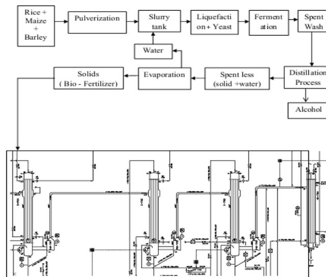
Fig. 1 Process Layout of Distillery plant
