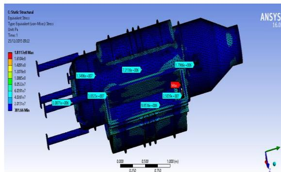
Fig.6 Steady state equivalent stress for shell
