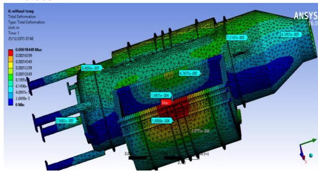
Fig. 4 Total Deformation for 5 mm shell wall thickness
